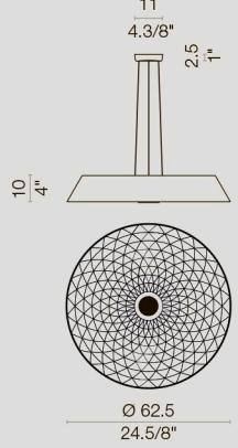
[En] → Flat panel glass front diffuser, with multi-layer silkscreened décor. Prismatic thermoformed PMMA side diffuser, detail in carved solid aluminium, chrome or polished gold, white ceiling canopy.
